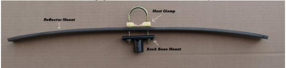
2 Slide the mast clamp / reflector arms onto a mast, and center it on your reflector both vertically and horizontally. The center to center distance of the reflector arms / mast mounts should be about 18 <sup>3</sup>/<sub>4</sub>" to fit the supplied back bone PVC center piece but can be as much as 2" shorter if needed. Try to align the reflector mounts so that they line up with the horizontal running wires of the reflector if possible.
